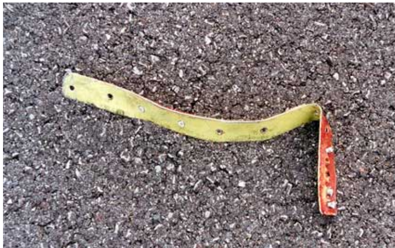
The plate that caused the tyre to explode
